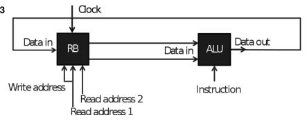
The ALU of the processor above has two instructions: 0 = `ADD' and 1 = `MUL'. Furthermore it has four 8-bit registers. Give for this processor the program for computing R1  $\times$  R2 + R1  $\times$  R3 + R1 and storing the result into R1. (You may not need all timeslots.)
