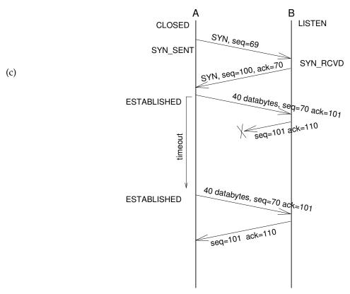
Note that the last packet from A is a retransmission (since it comes at the end of a timeout), not new data, hence the same sequence number.
