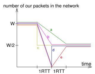
3 pt (c) Suppose we would like to follow the purple line (labelled b): the number of packets in transit gradually decreases during 1 RTT, and after 1 RTT, it stabilizes at half of the congestion window before the loss.
