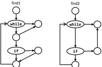
The **while**-condition in the first flow graph is split in two to faithfully reflect the behavior of the (conditional) &&. The complexity can for instance be computed as #edges - #nodes + 2; this yields
