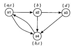
Four atomic propositions are used: a, b, c and d. Next to each state, the set of the atomic prositions is indicated that hold in that state.
