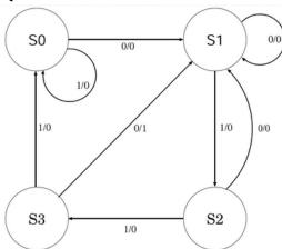
This finite state machine is realized with 2 data flip flops  $(Q_1Q_0)$   $(Q_1$  is the left bit of the state) and combinational logic. The input is X and the output is Y. The encoding of the states is:
