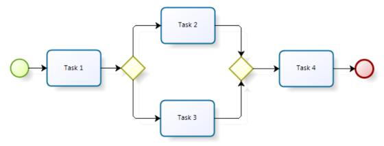
Suppose that the two gateways are of type AND. If 3 instances of this model are started at the same time, what can we say about their execution logs (keeping a record of the successfully executed tasks) before completion of any of the instances?
