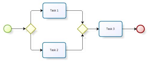
Suppose the split gateway is of type XOR and the join gateway is of type AND. If this process starts 6 times, how many times will either Task 1 or Task 2 be executed?
